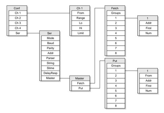
The menu is arranged hierarchically. The first level contains four submenus, one for each analog output, and a serial communications submenu. Some of the settings are hidden when they are not used.
