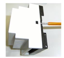
To set up the jumpers, the enclosure has to be opened. Detach the device from the DIN rail, and insert a flat bladed screwdriver between the black and grey parts of the enclosure and lever carefully.
