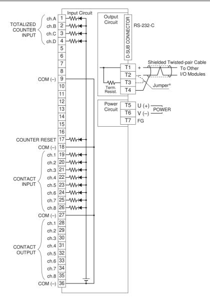
\* When the device is located at the end of a transmission line via twisted-pair cable, (when there is no cross-wiring), close across the terminal T2 –T3 with the attached jumper pin (or with a leadwire).
