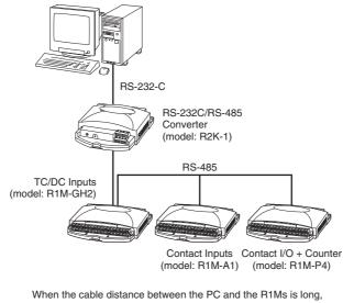
insert an RS-232-C/RS-485 Converter for isolation.
