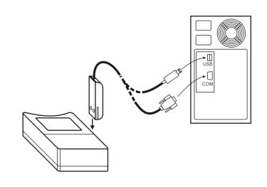
to use USB ADAPTER. Connect adapter connector to proper computer port and plug the adapter to the guide slots on the side of logger.
