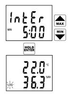
Now instrument displays adjusted storing interval. To modify the storing interval use arrow keys. Interval 10 sec is displayed as **MIN 0:10**, minute intervals are displayed as **MIN x:00** and hour intervals as **x:Ho**. Confirm adjusted interval by pressing ENTER key. Notice: if manual logging mode is selected, this menu item is skipped (there is no interval adjustment).
