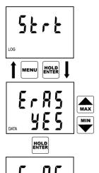
If it is needed to clear the memory before logging start, first it is necessary to select menu item logging START (symbol Strt) and confirm by pressing ENTER kev.
