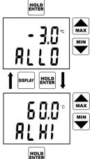
Reading ALLO indicates adjusted lower alarm limit (here air temperature). Set the desired value by means of the arrow keys. Press and hold the arrow key UP to make value increase fast. Press and hold the arrow key DOWN to make value decrease fast. Release the arrow key and press ENTER to confirm new limit
